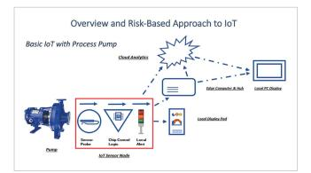
Simple list of typical parts of a wireless IoT system in a fluid handling process. Image courtesy of Tom Meir, M E I R Consulting, Pump Knowledge Workshop Instructor.
